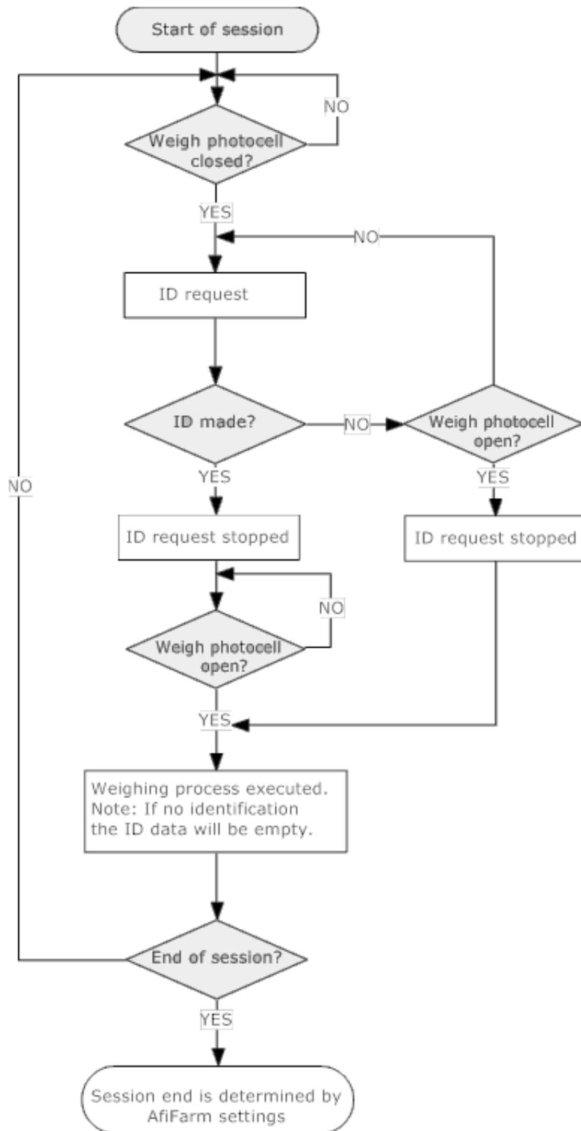
**Figure 34: Weigh System Operation Sequence**
