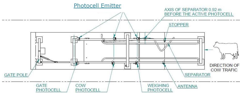
**Figure 15: Separator Sort & Weigh Station**
