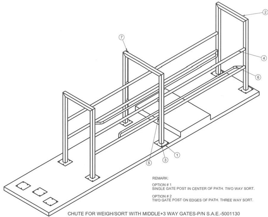
**Figure 4: Chute with 3 Way Exit**
