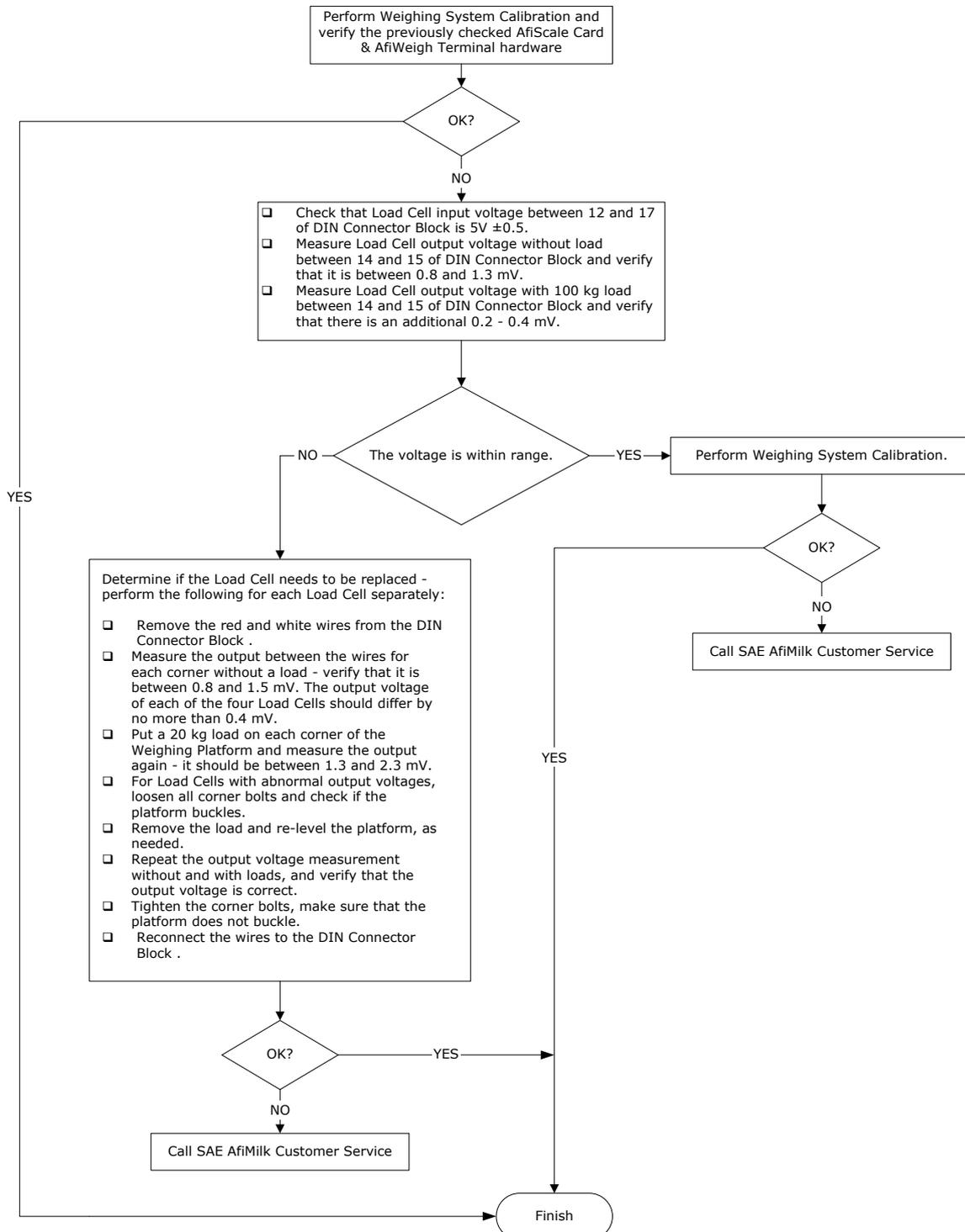
Figure 40: Load Cell Malfunctions Troubleshooting Procedure
