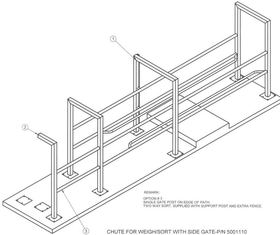
**Figure 5: Chute with Two-Way Exit**
