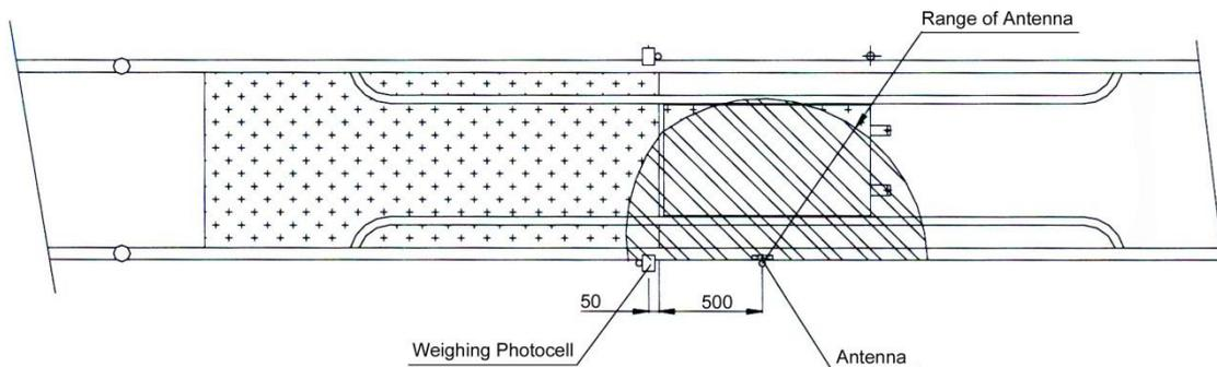
**Figure 32: Testing Antenna Range for Combined AfiSort/AfiWeigh**
