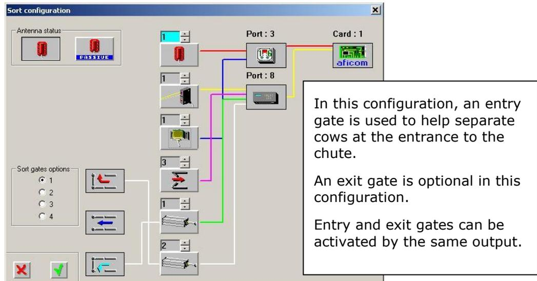
**Figure 31: Sort Configuration with an Entry Gate (with a gate limit switch to indicate gate closure)**
