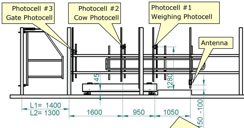
Distance between antenna and photocell *depends on the leg carrying the tag* (see Figure 14)
