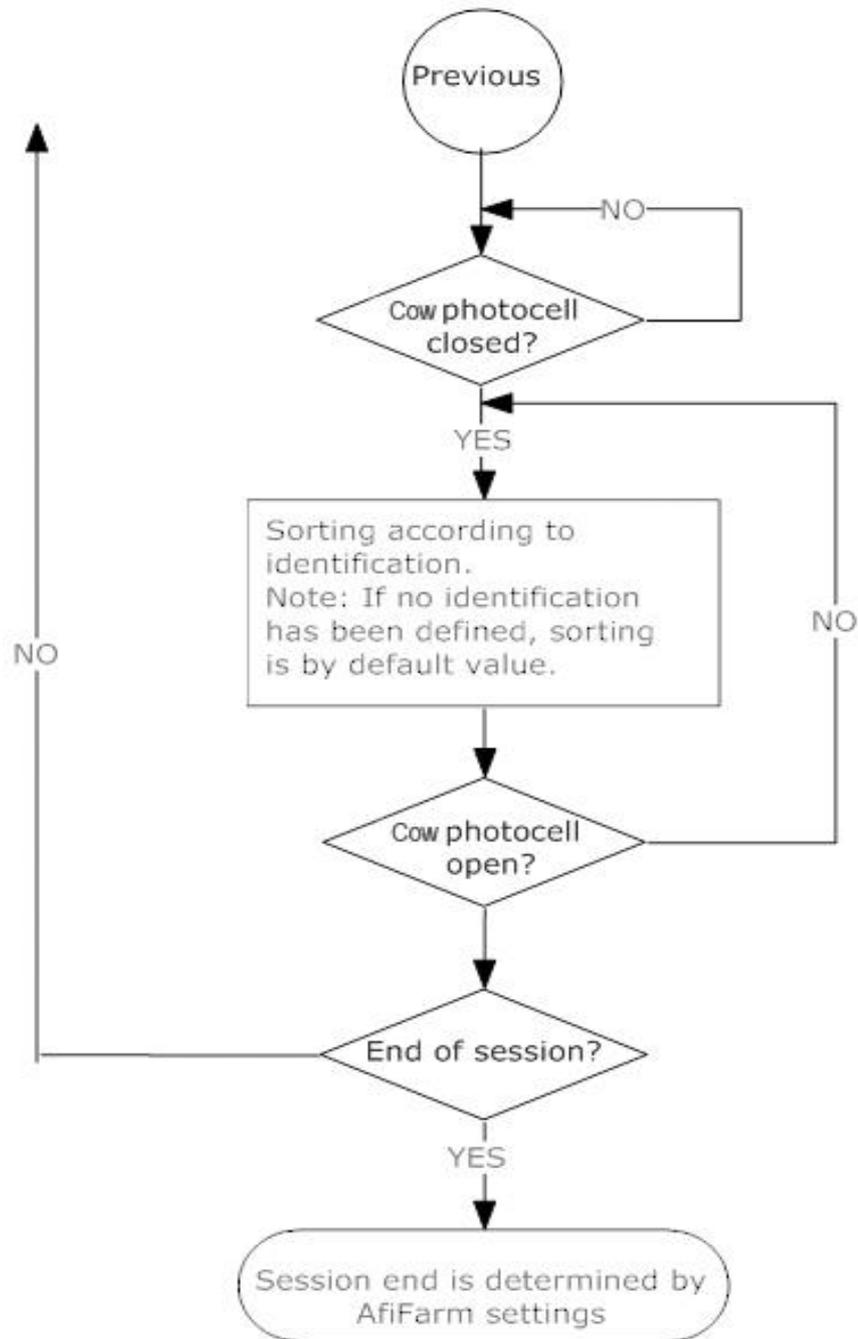
**Figure 35: Weigh and Sort Operation Sequence**
