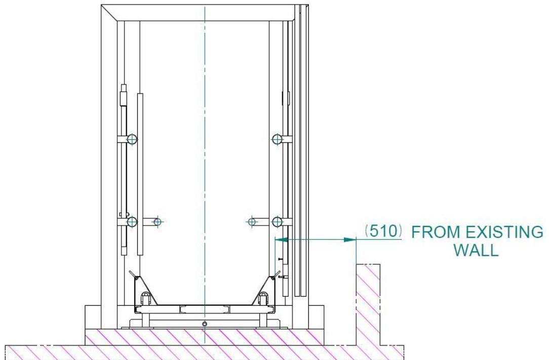
**Figure 7: Minimum Distance from Wall**
