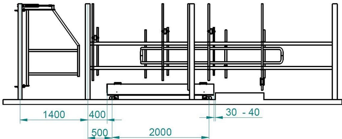
**Figure 9: Weigh Station—Plan Side View**
