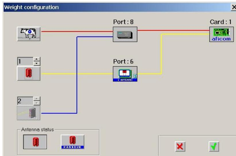
**Figure 28: Walkover Weight Configuration Screen - 2 Antennas Definition**
