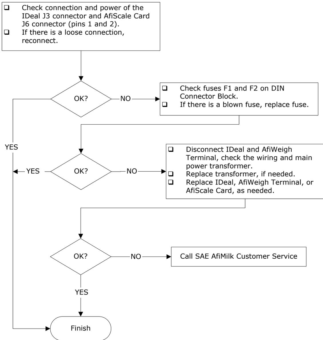
**Figure 36: System Power Check Procedure**
