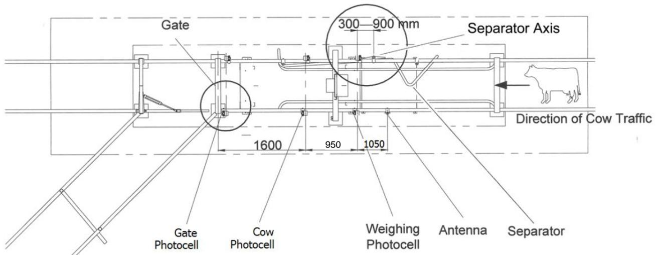
**Figure 19: Components of Combined AfiSort/AfiWeigh**
