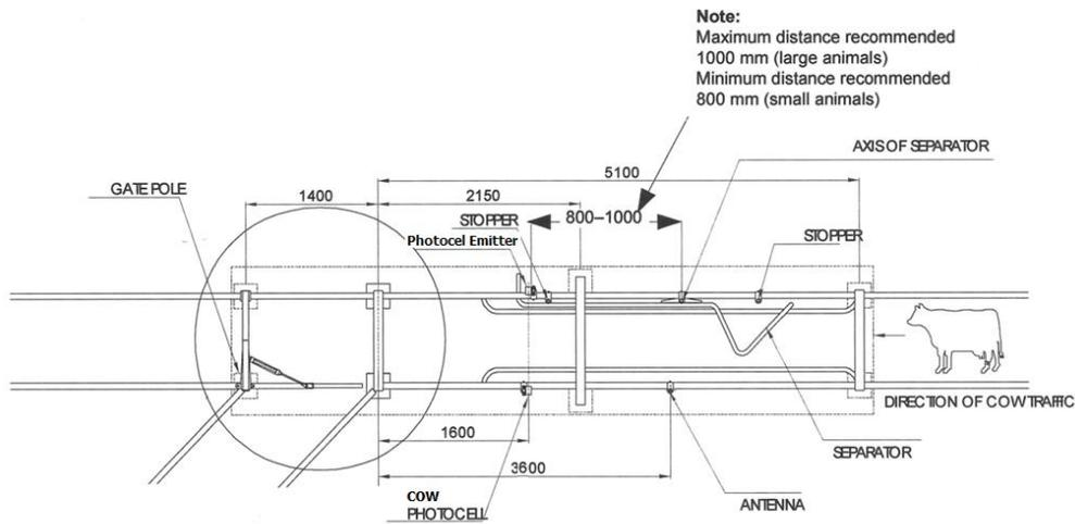
Figure 18 shows the components of AfiSort including the position of the Separator.
