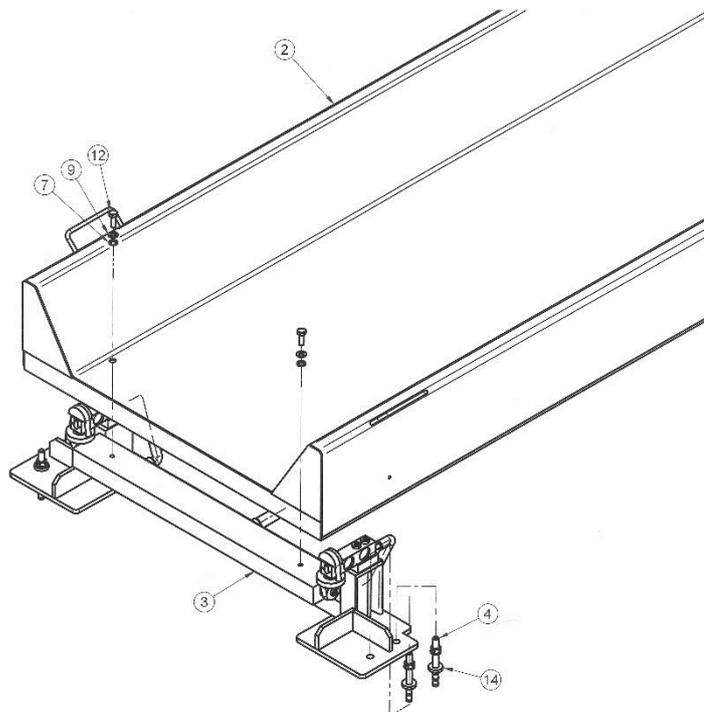
**Figure 10: Weigh Station – Assembly**
