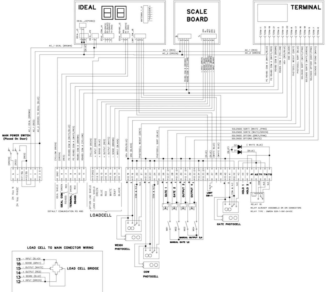
**Figure 21: Internal Electrical Connections Weighing & Sorting.**
